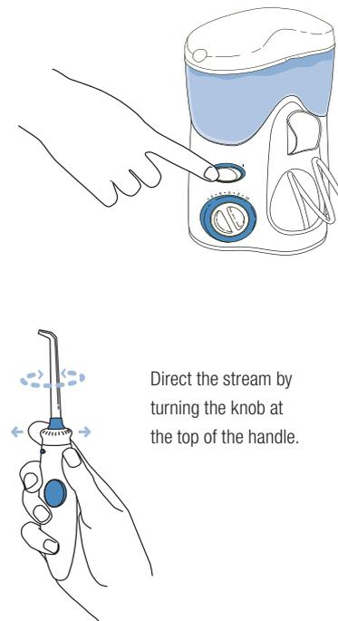
Direct the stream by turning the knob at the top of the handle.
